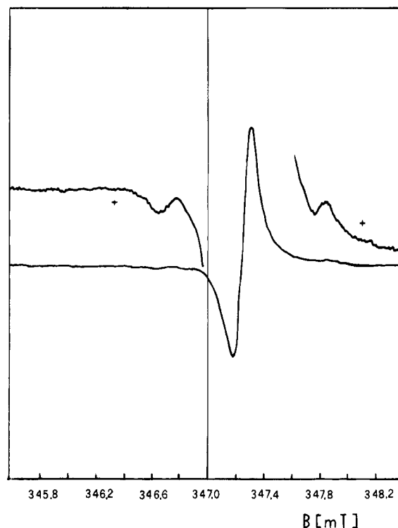
Figure 4. ESR signal of pristine powder of C_{60} . The trace marked + shows the lateral symmetric components at a higher gain ( \times 10 ) of the spectrometer. The splitting between the lateral components is 2D = 1.1 mT.
